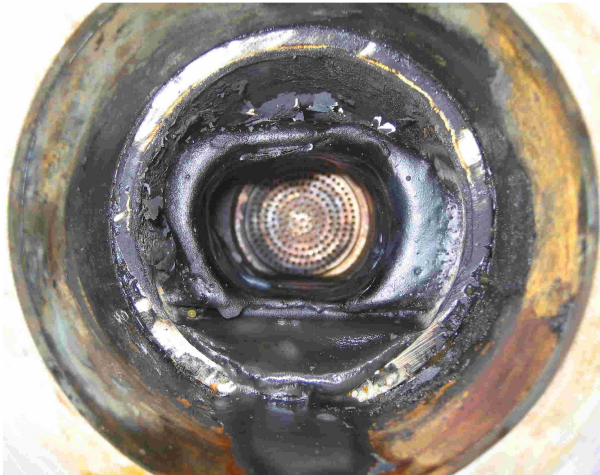
Figure 6. Paraffin fuel after firing.
