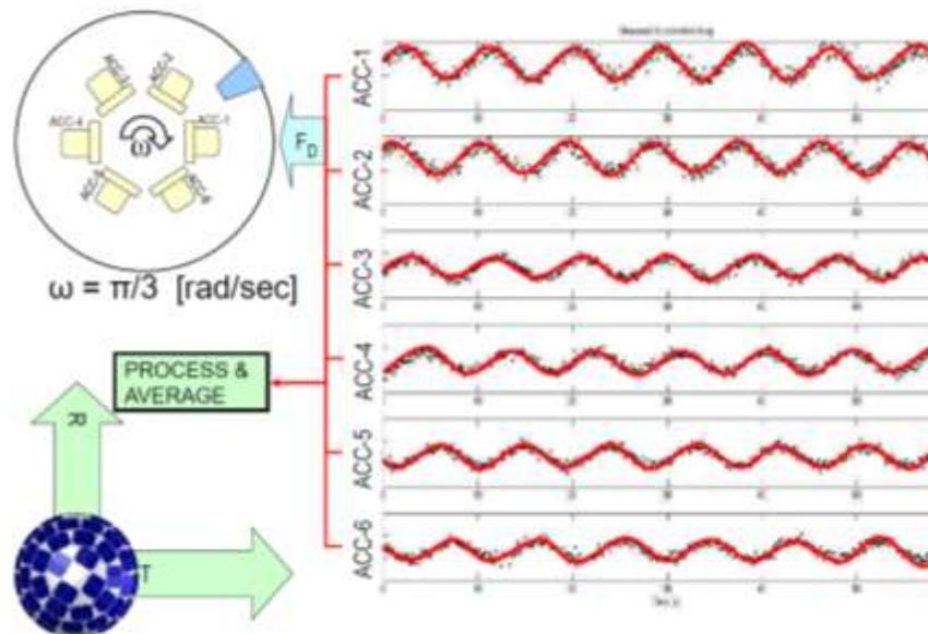
**Figure 2 DANDE Accelerometer System Measurements**
