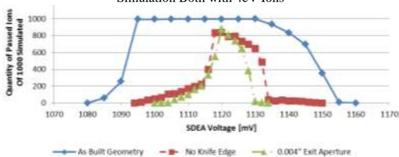
**Figure 9 Knife Edge Effects On Pass Band Geometry**
