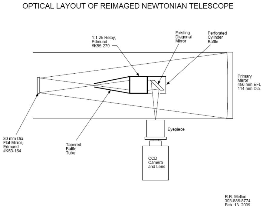
Figure 6: This drawing shows the optical layout for BOWSER's modified Newtonian Telescope, designed to baffle stray light to achieve images of stars from Earth's stratosphere during the day.
