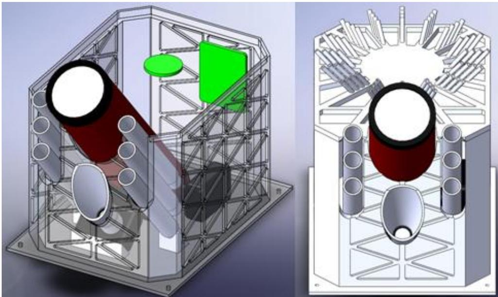
Figure 4: The two drawings show the preliminary design for the BOWSER payload. Notice the camera mounted for a wide angle view directly below the narrow telescope field of view
