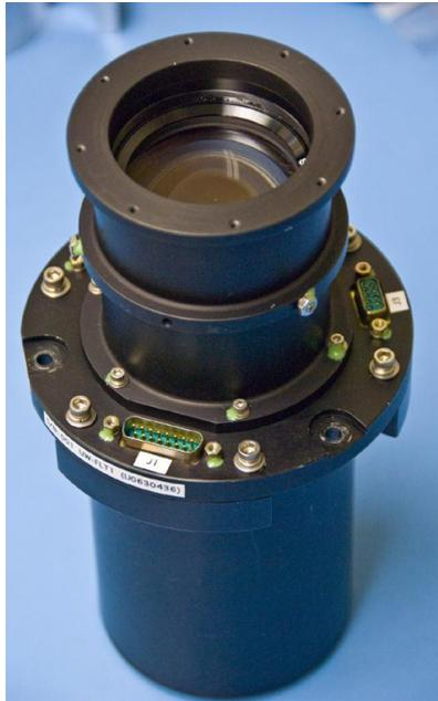
Figure 2: The ST5000 is making strides in improving the attitude determination, mapping and imaging of stars from sounding rockets, satellites, and balloons.
