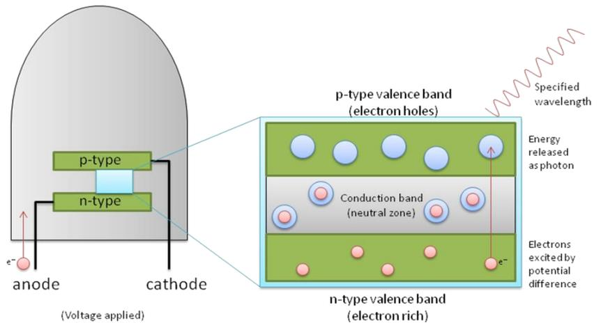
Figure 5: This diagram represents the functionality of an LED in the forward direction.
