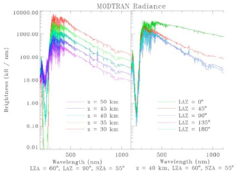
Figure 3: The MODTRAN model displays sky background as a function of wavelength, altitude, and angle from the sun.
