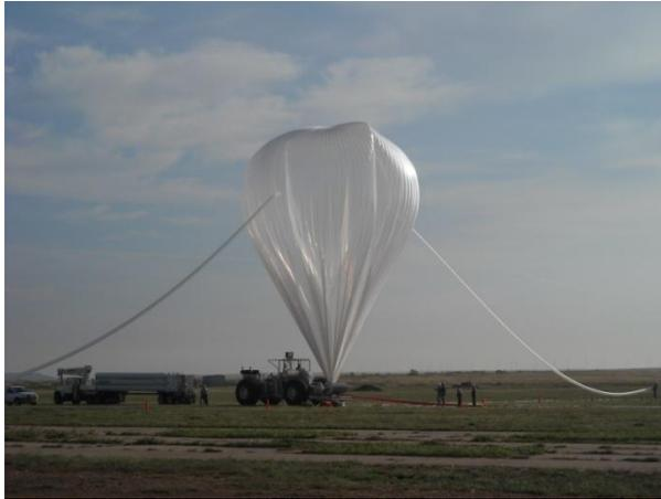
Figure 3: HASP balloon being filled prior to launch
